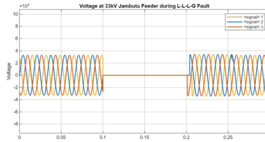
Figure 17. Voltage Waveform – L-L-L-G Fault
